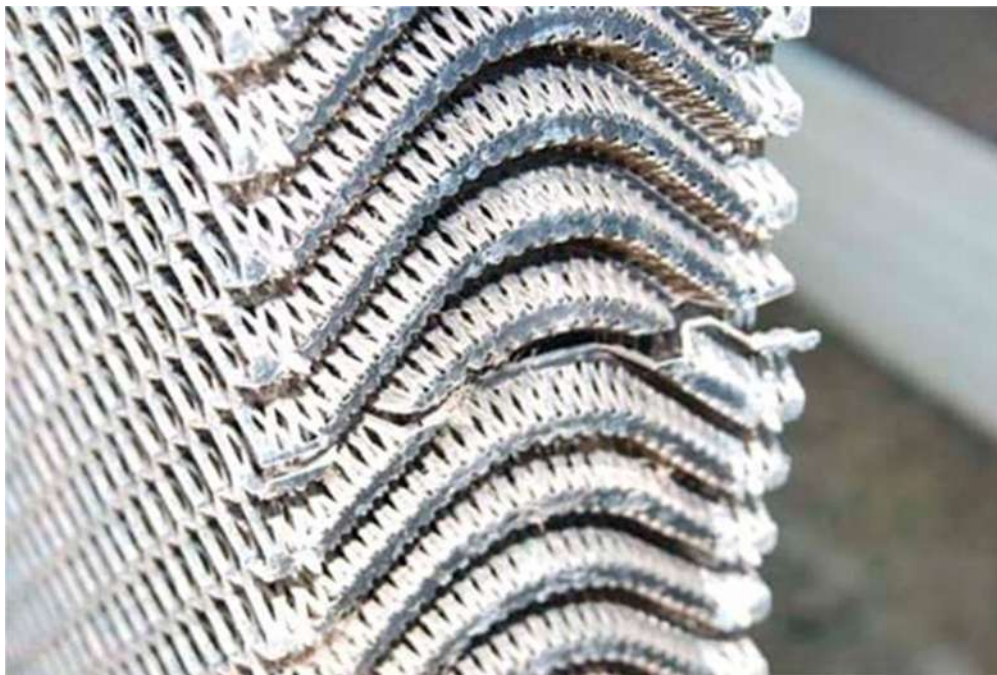
Figure 11. Unglued piece of plastic pad
