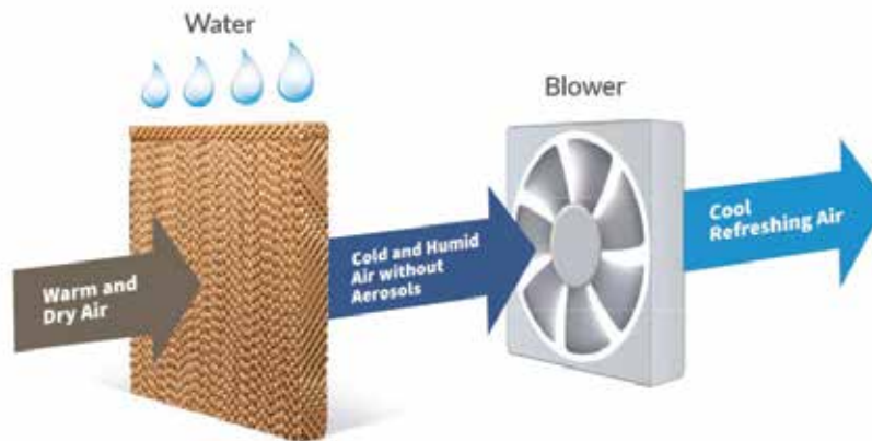
Figure 1: Cellulose pad in evaporative cooling system
